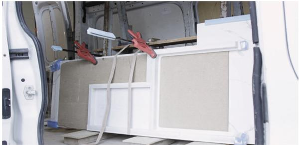
C) Secure the load with wood or ratchet straps. Ensure that the product is held firmly, without over tightening.
