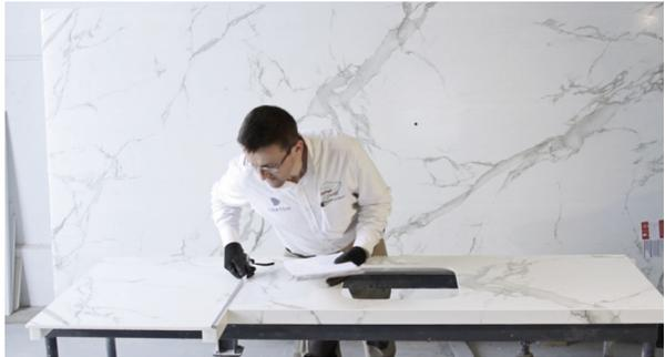
For pieces with large cut-outs, it is advisable to use fixation bars to prevent movement and breakage.
